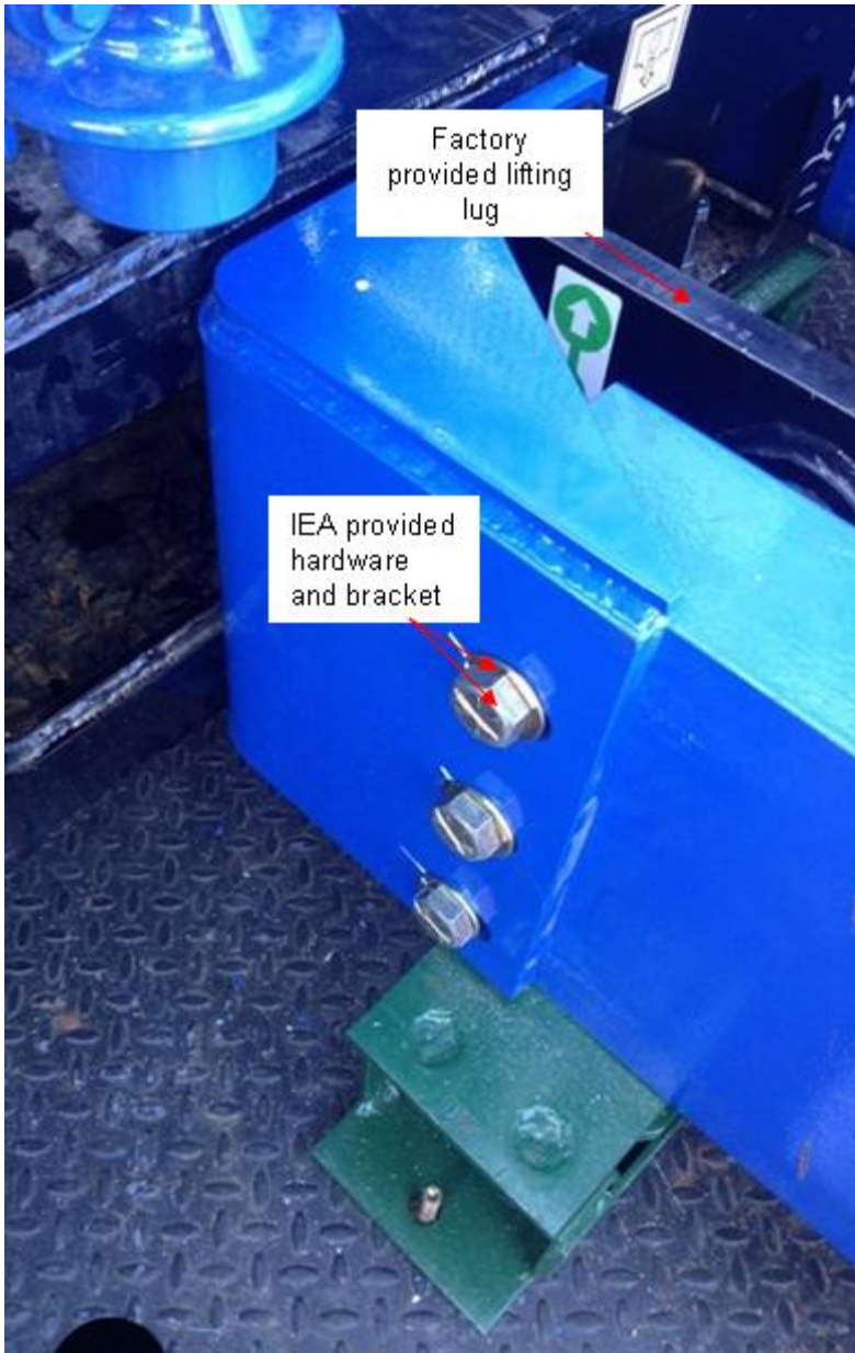
Figure 12: Engine rail to wishbone interface (outside view)
